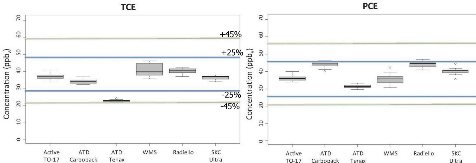
Results only for the center-point tests (all factors at middle of ranges)
