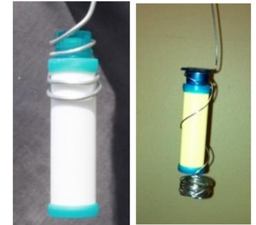
Limited to 1-inch diameter or less – Low-Uptake Rate Samplers
